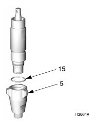
**8.** Disassemble intake valve. Be sure to remove o-ring (10).
