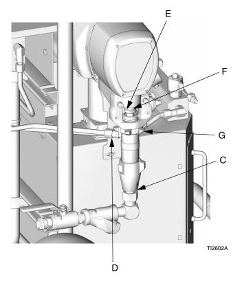
Fig. 1. Disconnect Pump (Pump A Shown)
