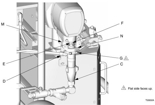
Fig. 2. Reconnect Pump (Pump A Shown)
