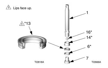
Sealing patch on piston threads is good for four repackings. Use Loctite® on piston threads after four repackings; be sure none gets on ball.
