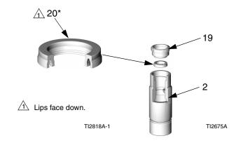
Model 245970: Grease u-cup (20\*) and cylinder (2). Place seal installation tool (23\*) in cylinder. Place u-cup in tool with lips facing down. Be careful not to damage sealing edges of u-cup. Press u-cup in place with 7/8 in. deep-well socket (S). Remove socket and tool.
